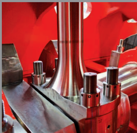
Hydraulic bolting on critical connections
