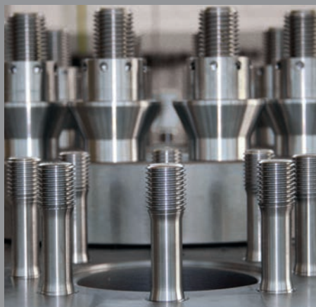
Stud bolts instead of cap screws
