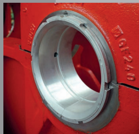
Vertical bearing split for increased reliability
