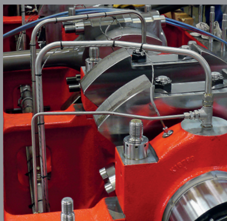
Stainless steel internal frame lube oil header and tubing
